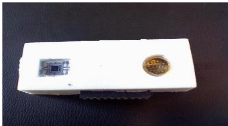
Figure 1.3 Wireless f NIRS device after packaging [10]
